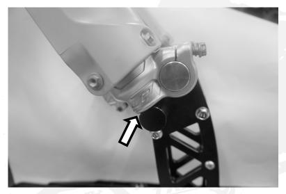
⇒ Confirm that the flats on the fork brace (FE) are sitting flat against the bottom of the fork tube with no space.
