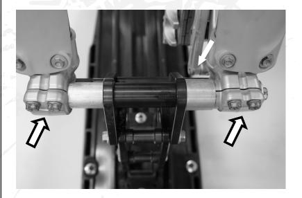
⇒ Now tighten the fork end bolts as and torque to the recommended value from the bike manufacture.
