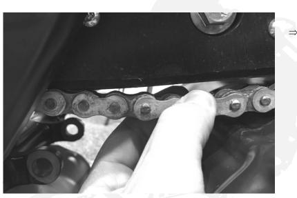
Spin the adjusting bolt counter clockwise to tighten the primary chain. The chain should be tight enough that you can only get 1/4"" to 1/2"" of play between the chain guide and chain if you are pulling down on it.
