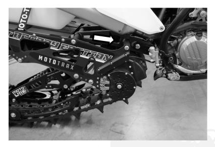
⇒ With help slide the kit into place as shown behind the bike. The more aligned the kit is at this step the easier it will be to mount the kit.
