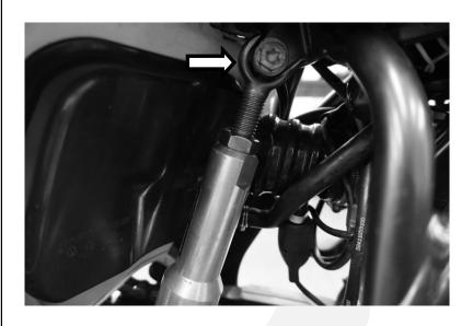
$\Rightarrow$  Mount the strut into the upper shock hole as shown, torque bolt to OEM specs.
