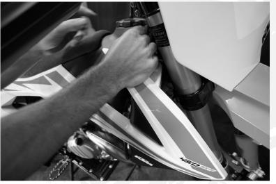
⇒ When routing through the steering head make sure that you turn the bars fully both directions and confirm that the line will not snag or kink on anything. Cable ties may and should be used to hold the line in place to prevent the line from shifting during use.
