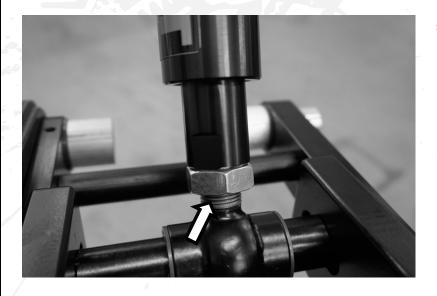
⇒ Spin the IDT strut (TB) onto the strut end as shown, leave about 1/4" of visible threads showing below the jam nut, securely tighten the jam nut at this point.
