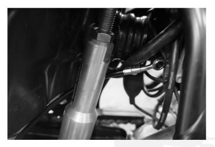
⇒ Route the brake line through the track system and around the strut as shown making sure it is clear of the drive chain, exhaust and anything else that my snag, tear, or burn the line and cause future failure.
