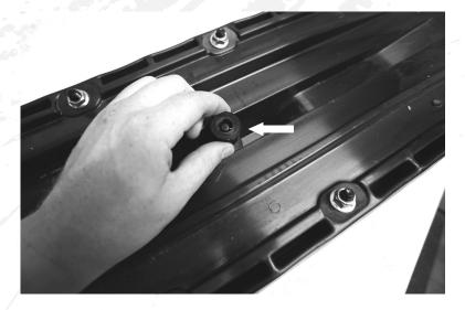
⇒ Now install spacer (CA) on the center mounted ski studs as shown.
