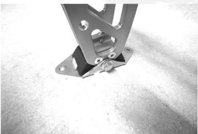
⇒ Than set the ski frame (SA) in the mount and secure with bolt and locknut (SB), make sure that the marks on the ski frame and the rubber damper line up.
