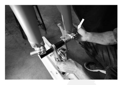
⇒ Take the ski axel bolt and large washer (DR) and insert from the caliper side all the way to the farthest fork bracket as shown.
