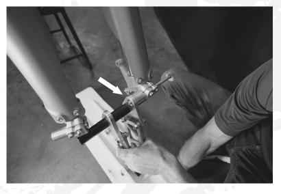
⇒ Now lift the ski frame assembly onto the spacer, note the square shapes need to line up.
